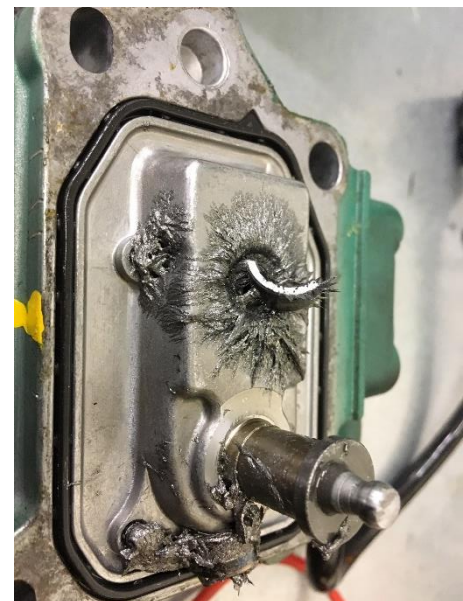
SWARF INSIDE FUEL INJECTION PUMP
