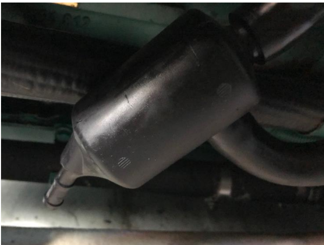
oil/air separator for crankcase rebreather
