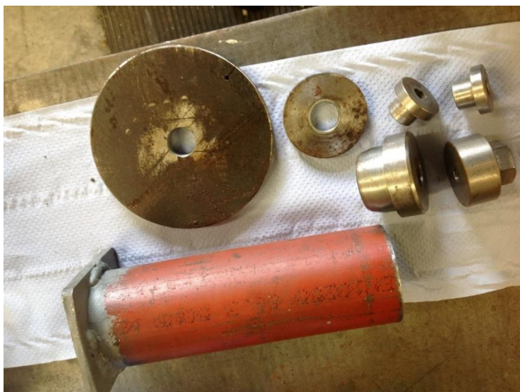
particularly happy with since the screws are merely tapped into the rather fragile fiberglass tube wall. Above shows the collection of parts I made to use with a length of 10mm screwed rod to enable removal of the two cutlass bearings.
